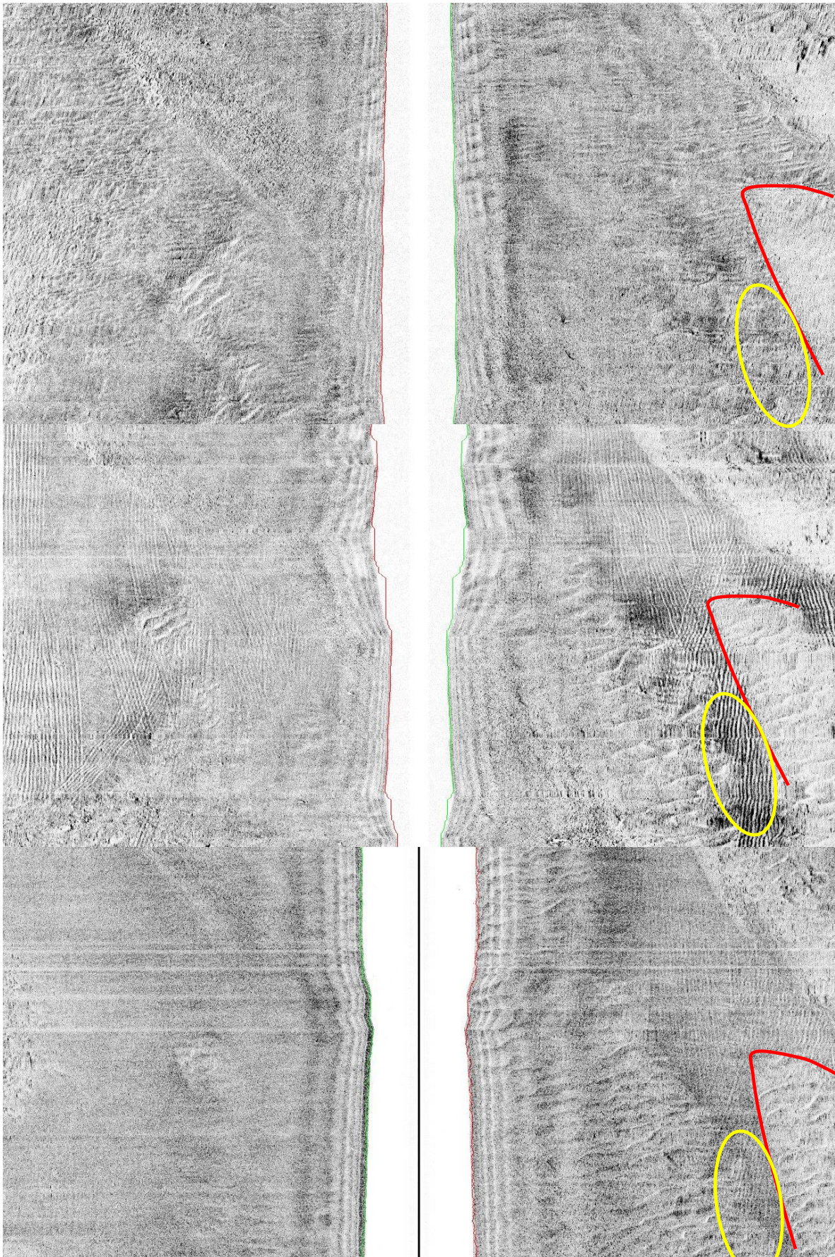
Figure 8 Side-scan sonar records from a section of Lane 12 (Fishing intensity: 2.29 times swept) in March 2014 (top), May 2014 (middle) and September 2014 (bottom). Red lines highlight some common features. Yellow lines highlight areas in which dredge marks were visible in May and September.
