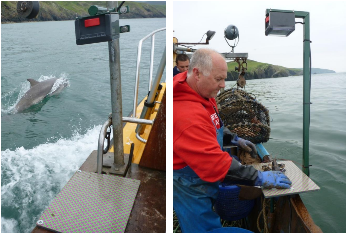
Figure 1. Camera system installed on board two fishing vessels, one operating off Hell's Mouth (Llyn Peninsula, North Wales) (left) and one fishing in Cardigan Bay (Mid Wales) (right). The square pattern measuring board is shown with the camera mounted in the grey box. The 'on/off' red switch is clearly visible to allow fishers to operate the system manually.
