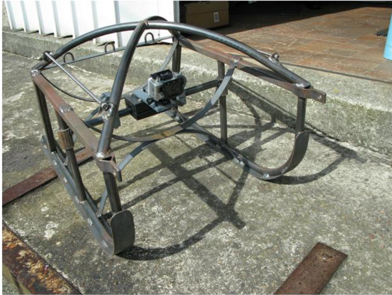
Figure 1. Mini-sled developed to be towed from fishers' vessels. Here, only mounted with GoPro video (laser pointers and lights were added later).
