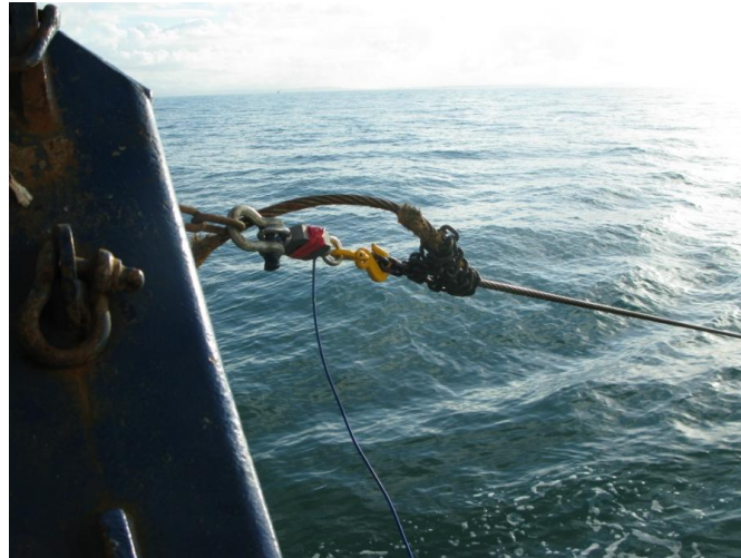
Figure 6. Load cell measuring tension on cable towing scallop dredges, as a proxy for fuel consumption.
