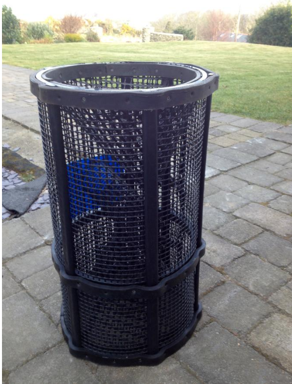
Figure 21. Roscoff-like prawn pot (made in Wales). Body and end mesh 8mm to retain all sizes.
