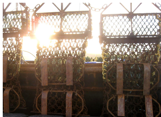
Image - Steel skids attached to scallop dredges (Harriet Salomonsen)
